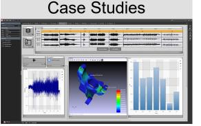
2015, **Time v Frequency Domain Analysis for Large Automotive Systems**, SAE Paper 2015-01-0535. Pioneering work done with **Booz Allen Hamilton** on fatigue of large automotive system (truck cab) done in both the time and frequency domain.
