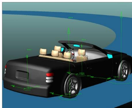
**Cornering events:** Investigate both steady-state and limit cornering to capture responses such as understeer/oversteer gradients
